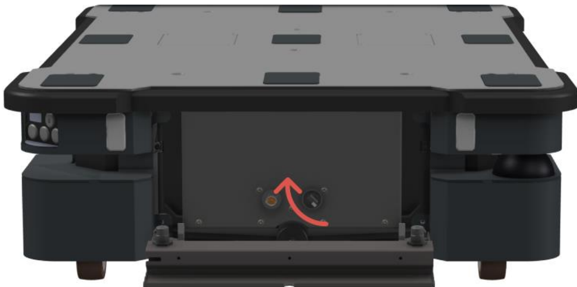
Figure 5.4 Turn the Manual brake release switch clockwise to release the brakes
