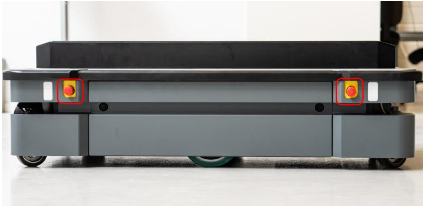
Figure 5.2 MiR600 has four Emergency stop buttons: two on each side of the robot
