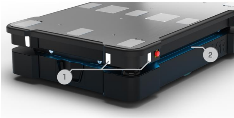
Figure 4.1 Light indicators on MiR1350
