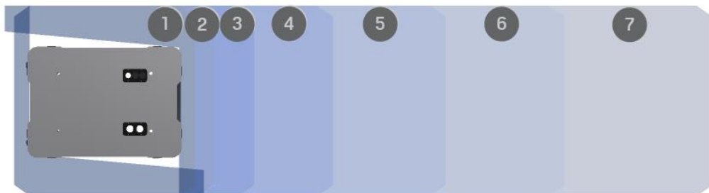
Figure 9.3. The illustration shows the field set contours when driving forward. The range of the field set changes with the robot's speed.
