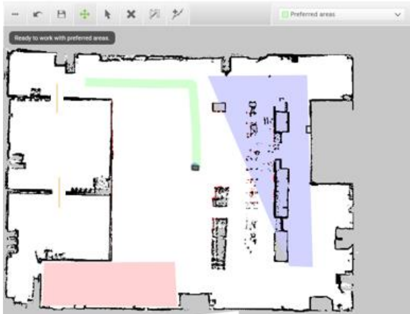
Figure 10.1. Unpreferred zones (marked with purple) can be used in highly dynamic areas to solve issues with re-planning of paths.
