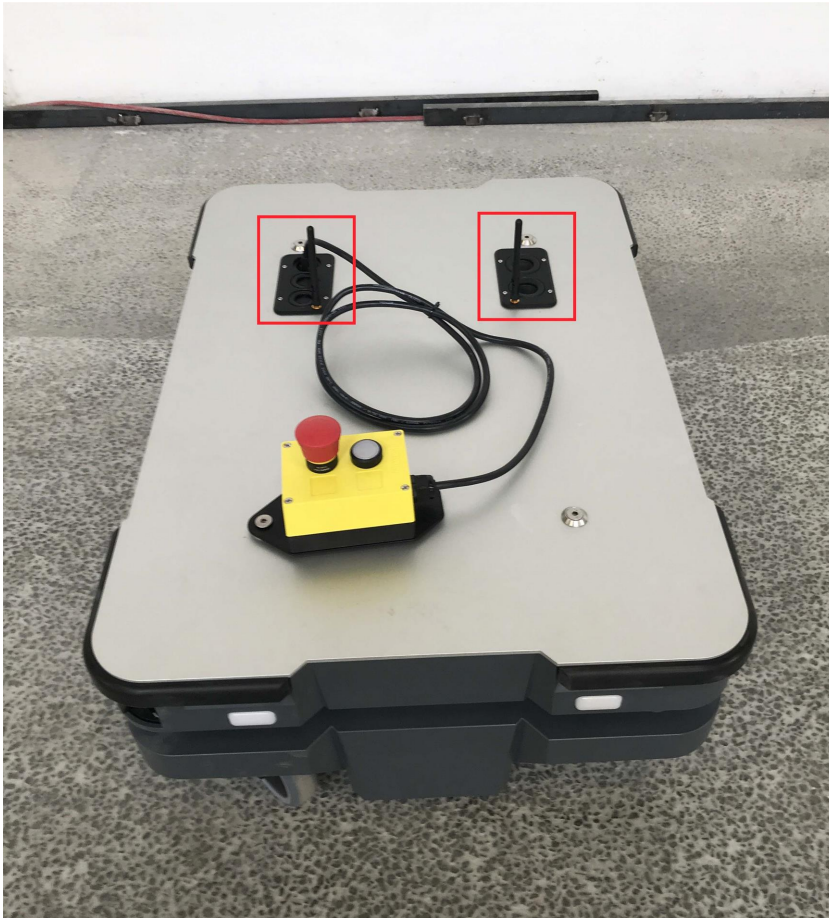
Figure 5.1. The top compartments of MiR250.
